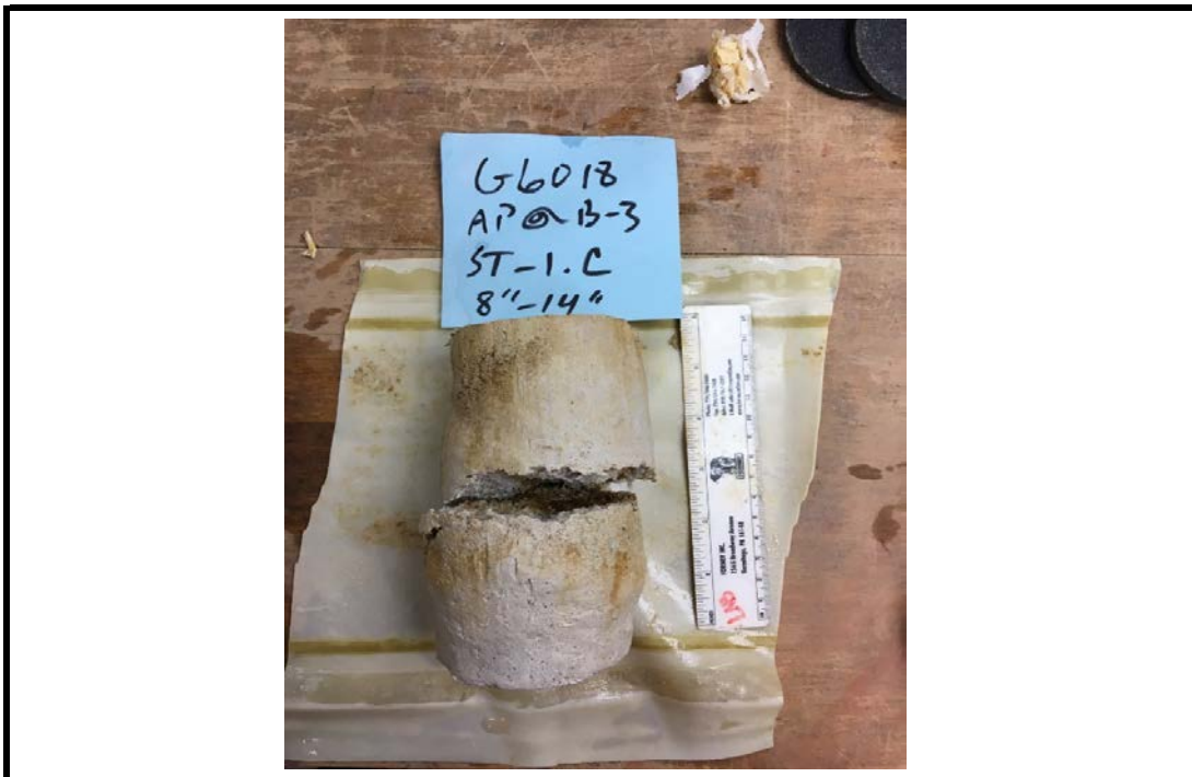
Specimen No. ST-1.C Photo 2 (After CU Testing)
