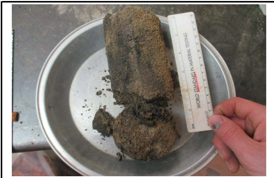
Specimen No. ST-1.A Photo 2 (Collapse)
